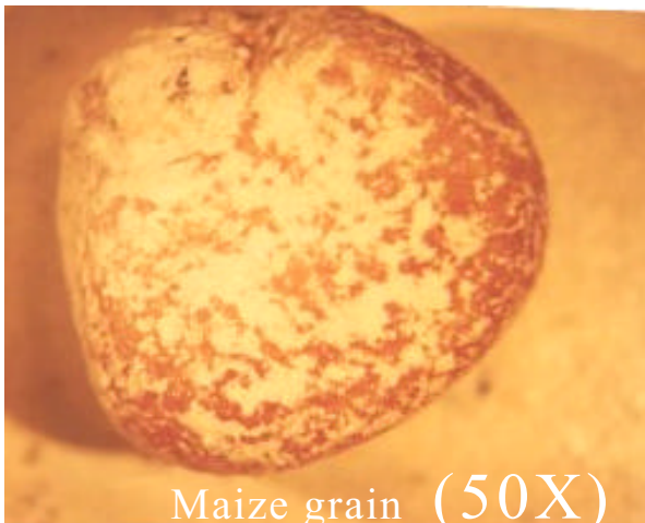
c) NeemAzal ® coating on a grain treated with the product
